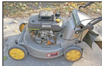
John Deere 14SD self propelled mower 5½ hp, 5 speed, 21" cut
